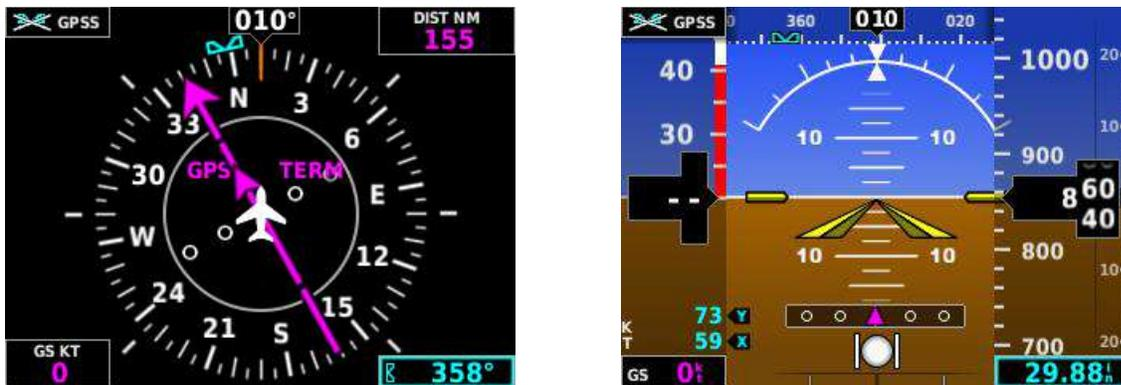
When GPSS is selected on the G5, GPSS turn commands are converted into a heading error signal to the autopilot. When the autopilot is operated in HDG mode, the autopilot will fly the turn commands from the GPS
