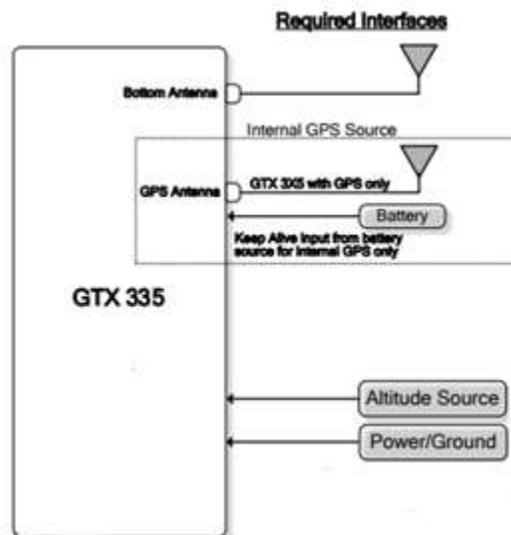
**Figure 1 – GTX 335 W/GPS ADS-B Interface Summary**
