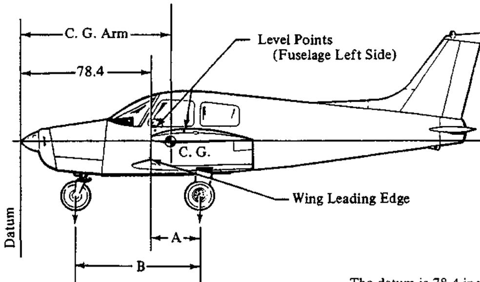
The datum is 78.4 inches ahead of the wing leading edge at the intersection of the straight and tapered section.
