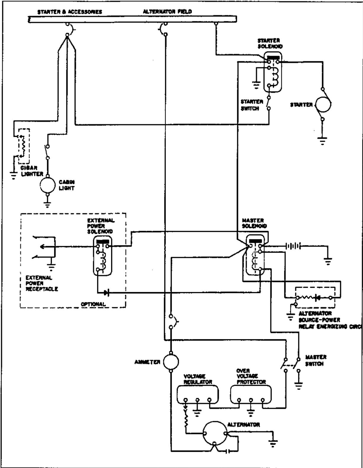
Alternator and Starter Schematic (Ser. nos. 7425001 through 7425454)
